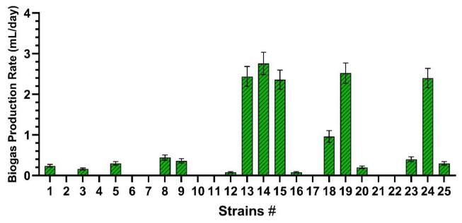
Fig. 1. Biogas production rate of different yeast strains over 5 days. Values represent mean ± SD.
