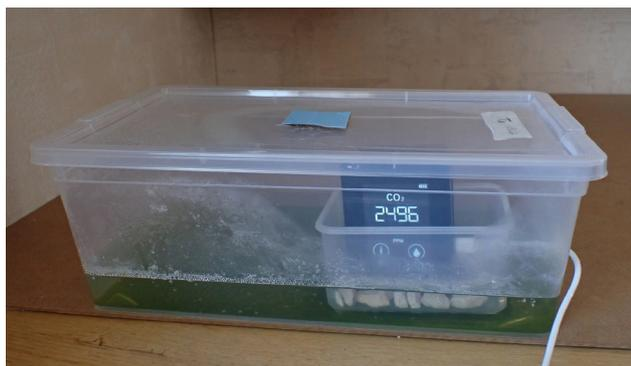
**Fig. 4.** Experimental device used to measure the carbon dioxide released by the water, inorganic fertiliser alone (IF) and inorganic fertiliser + algae (IF + A) treatments. Temperature (in °C) and hygrometry (in % relative humidity) were recorded at 9:00 and 21:00 (© Frédéric Darriet).
